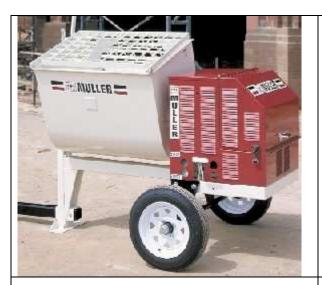
A Motor mixer like the one in the Picture should be acquired with an electric motor. The RPM's that the mortar mixer normally runs at for cement mixes is too fast for our purposes (because mortar is more liquid) and must be changed to work at 40-50 RPMs for the filter mix which is much more dense and "sticky".
