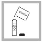
7. Fill another cell with 10 mL of sample (the blank). Wipe off any fingerprints or liquid.
