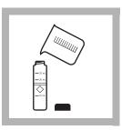
**6.** Fill a sample cell with at least 10 mL of sample (the blank).
