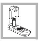
7. When the timer beeps, place the blank in the cell holder. Tightly cover the sample cell with the instrument cap.
