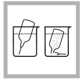
6. Prepare the sample: Collect at least 40 mL of sample in a 50-mL beaker. Fill the AccuVac Ampul with sample. Keep the tip immersed while the Ampul fills completely.
