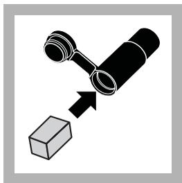
**5.** Prepare the calibration and storage chamber by holding it under water and squeezing it a couple of times to pull water into the lower chamber through the inlet.
