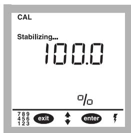
**14.** Press the **READ/ENTER** key. The stabilizing icon will appear while the meter completes the calibration.
