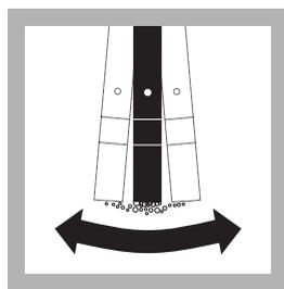
**19.** Agitate the probe in the sample to dislodge air bubbles from the sensing area of the probe tip.
