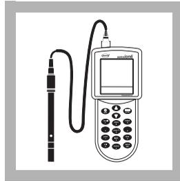
**2.** At least one hour before measurement, polarize the probe by connecting it to the meter. See *Section 3.3.2 Probe Polarization*.
