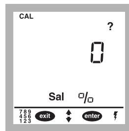
**12.** Since this calibration is performed in water saturated air, set the salinity to zero. If necessary, use the keypad to enter a salinity value of **0 0/00**.
