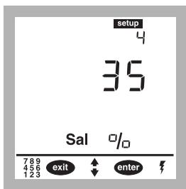
**17.** If sample salinity has been measured using an Electrolytic Conductivity Meter, enter the value in setup 4.
