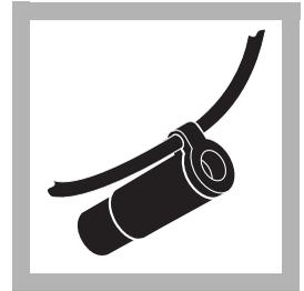
**4.** Secure the probe cable to the calibration and storage chamber by wrapping cable through the bottom of the chamber lid before filling with water.
