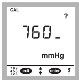
**9.** The main display will show the current value for the barometric pressure. If the meter has been moved to a different elevation or if the barometric pressure has changed, enter the new value. See Table 5 on page 63.
