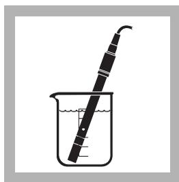
**18.** Insert the probe into the sample. The probe must be deep enough to cover the thermistor (metallic button) located on the side of the probe.
