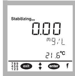
**3.** Zero the *sens<sup>ion</sup>™6* Dissolved Oxygen meter prior to calibration when measuring dissolved oxygen levels less than 1 mg/L or 10% saturation.
