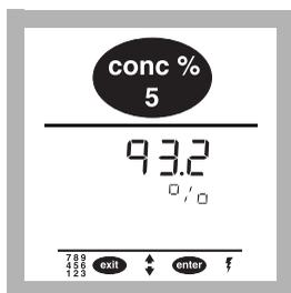
**22.** Press the **CONC %** key on the keypad to change the display from concentration in mg/L to % saturation.
