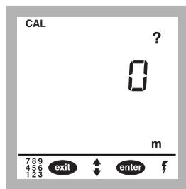
**11.** When the altitude is correct in combination with the barometric pressure press the **READ/ENTER** key. The current value for the sample salinity (0/00) will be shown.
