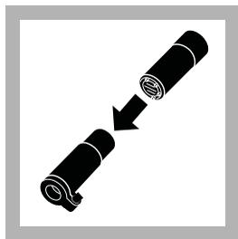
**6.** Insert the DO probe into the calibration and storage chamber. The probe tip must not be flooded with water or be holding a drop of water on the membrane.
