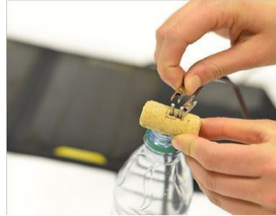
Fig. 11. Attaching electrical leads of solar panel.
