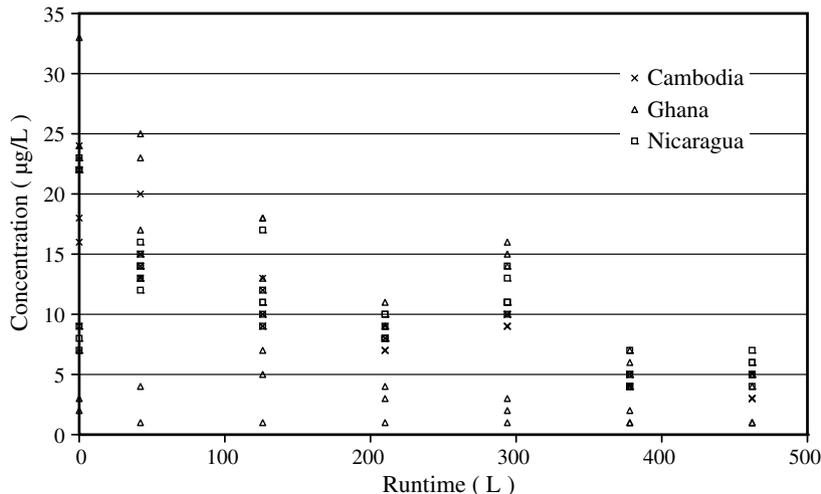
Fig. 3. Leaching of silver from the filter material of 6 filters per manufacturing location. Total filter runtime is 12 weeks, with a production of 6 L per day.
