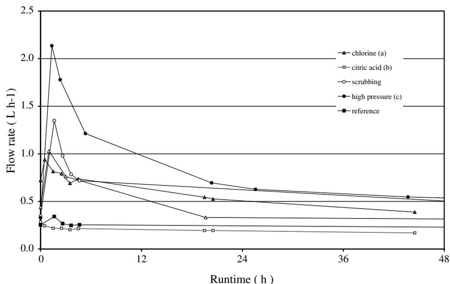
Fig. 5. Flow rate during first 48 h after scrubbing, citric acid (a), chlorination (b), high pressure (c), or with water pre-treated by sand filter.
