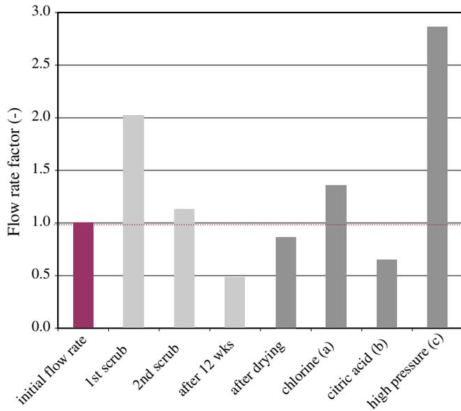
Fig. 4. Flow rates in relation to the initial flow rate (=1.0).
