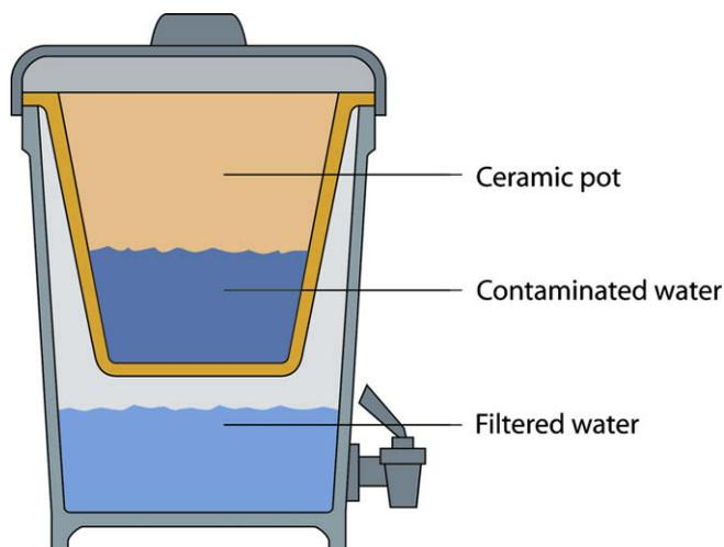
Fig. 1. Ceramic silver-impregnated pot filter (CSF).
