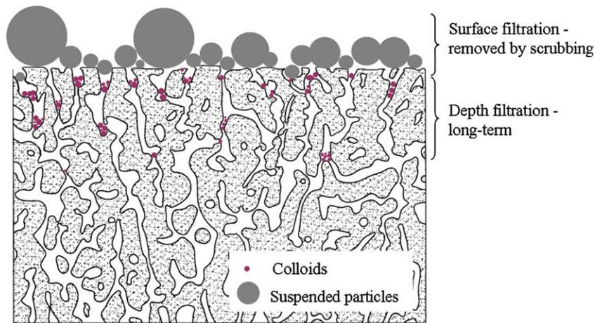
Fig. 6. Diagram of the hypothetical surface and depth filtration by suspended particles and colloids in CSF.
