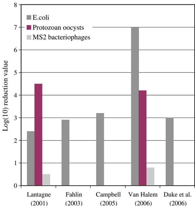
Fig. 2. Overview of the removal efficiency of *E. coli*, protozoa oocysts, and MS2 bacteriophages by the Nicaraguan ceramic silver-impregnated pot filter.
