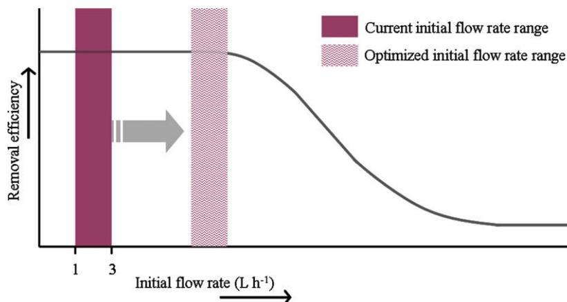
Fig. 7. Probable relation between removal efficiency and initial flow rate of CSF.
