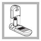
**8.** Immediately place the prepared sample into the cell holder. Tightly cover the sample cell with the instrument cap.
