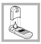
**8.** Immediately place the AccuVac Ampul into the cell holder. Tightly cover the ampule with the instrument cap.
