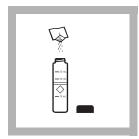
7. Add the contents of one DPD Free Chlorine Powder Pillow to the sample cell (the prepared sample). Cap the cell and swirl vigorously to dissolve the powder.
