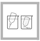
**6.** Fill a DPD Free Chlorine Reagent AccuVac Ampul with sample.
