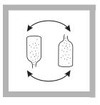
**7.** Quickly invert the ampule several times to mix. Wipe off any liquid or fingerprints.
