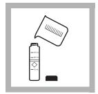
**3.** Fill a sample cell with 10 mL of sample (the blank).
