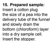
The lead-dithizone complex is stable for at least thirty minutes if the sample cell is kept tightly capped and out of direct sunlight.
