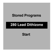
**1.** Select the test. Insert an adapter if required (see *Instrument-specific information*).
