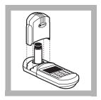
**8.** Place the blank into the cell holder. Tightly cover the sample cell with the instrument cap.
