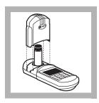
7. After the timer beeps, place the blank into the cell holder. Tightly cover the sample cell with the instrument cap.
