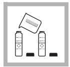
**3.** Fill two sample cells with 10 mL of sample each. One cell will be the prepared sample, the other is the blank. Set the blank aside.
