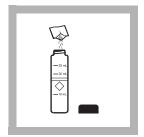
**4.** Add the contents of one NitraVer 5 Nitrate Reagent Powder Pillow to one cell (the prepared sample). Cap the cell.
