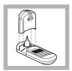
**9.** Place the AccuVac ampul into the cell holder. Tightly cover the sample cell with the instrument cap.
