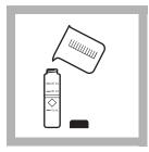
**6.** Fill a sample cell with at least 10 mL of sample (the blank).
