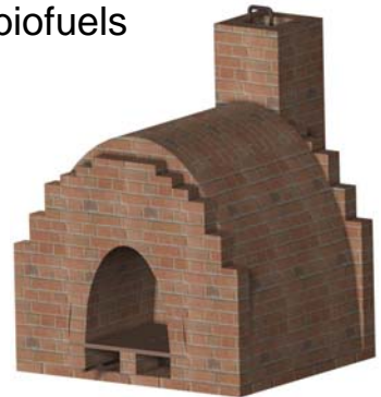
A downdraft, catenary arch style kiln was used for efficiency and ease of construction.
