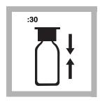
**5.** Place an ampul cap securely over the tip of the ampul. Shake the ampul for about 30 seconds. Wipe off any liquid or fingerprints.
