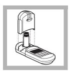
9. After the timer beeps, place the prepared sample into the cell holder. Tightly cover the sample cell with the instrument cap.
