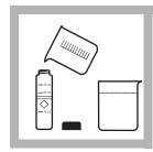
3. Fill a sample cell (the blank) with at least 10 mL of sample. Collect at least 40 mL of sample in a 50-mL beaker.
