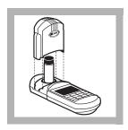
7. Place the blank into the cell holder. Tightly cover the sample cell with the instrument cap.
