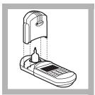
**9.** After the timer beeps, place the AccuVac ampul into the cell holder. Tightly cover the ampul with the instrument cap.
