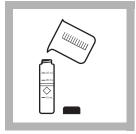
**6.** Fill another sample cell with 10 mL of sample (the blank).
