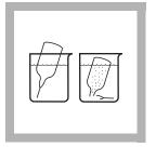
**4.** Fill a PhosVer 3 Phosphate AccuVac Ampul with sample.
