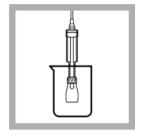
8. Put the electrode in the sample and press READ. For faster response, stir at a slow to moderate rate.
