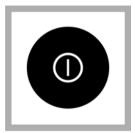
3. Turn the meter on. Make sure that the meter is set to measure to measure pH.
