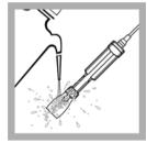
7. Rinse the electrode in deionized water and blot dry prior to sample measurement. Rinse the electrode between measurements to minimize contamination.
