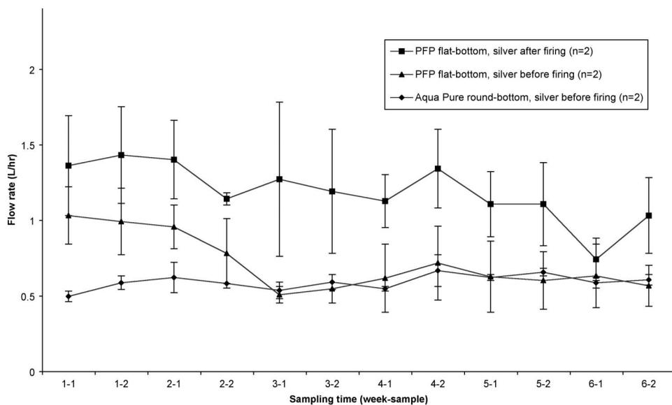
Figure 3. Flow rate in six filters of three types over 6 weeks.
