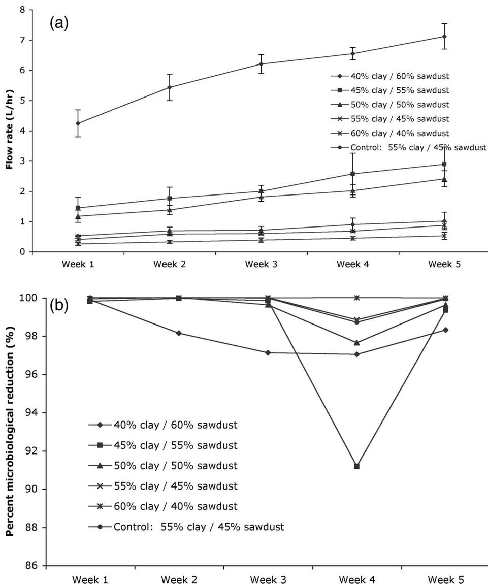
Figure 5. (a) and (b) Flow rate and total coliform percentage reduction in clay:sawdust ratio testing filters. Note: Results presented are averages of triplicate samples.
