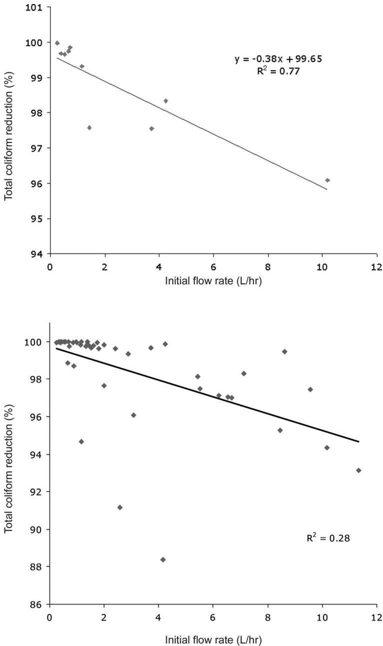
Figure 8. Regression analysis – percentage total coliform removal and flow rate (weekly per filter type [50 data points] and study average per filter type [10 data points]).
