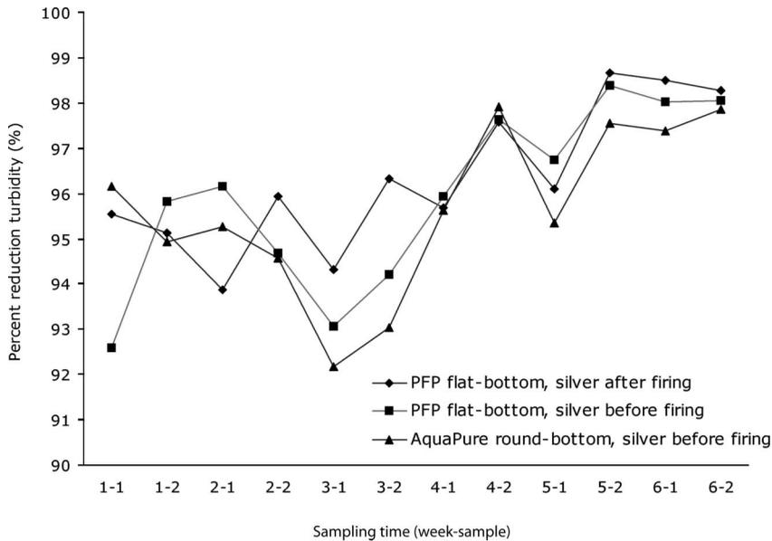
Figure 4. Percentage turbidity reduction of three filter types over 6 weeks. (Note:  $n = 6$  for each sample (duplicate filters with triplicate turbidity measured.) Errors bars not presented because y-axis is percent reduction, not NTU).
