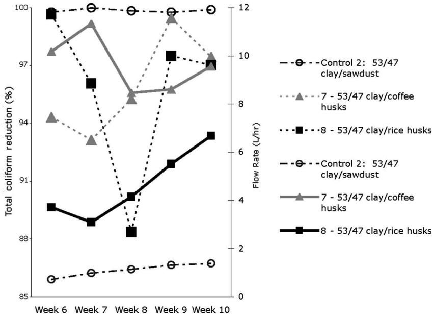
Figure 6. Flow rate and total coliform percentage reduction in burnable testing filters. Note: Dotted lines are total coliform reduction, solid flow rate, dashed control filters. Results presented are averages of triplicate samples.
