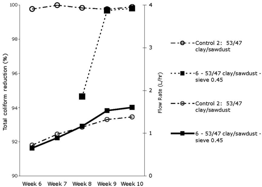
Figure 7. Flow rate and total coliform percentage reduction in sieve testing filters. Note: Dotted lines are total coliform reduction, solid flow rate, dashed control filters. Results presented are averages of triplicate samples.
