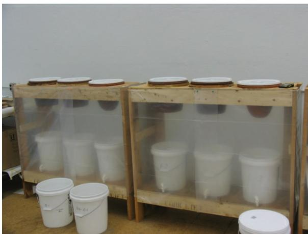
Figure 2. Laboratory set-up for filter testing at Lehigh University.
