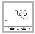
**15.** When the calibration is complete, the meter will return to the Reading mode. Press the **EXIT** key during the calibration sequence to back out of the calibration routine, one-screen-at-a-time, without completing a calibration.
