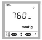
**9.** The main display will show the current value for the barometric pressure. If the meter has been moved to a different elevation or if the barometric pressure has changed, enter the new value. See *Table 5* on page *63*.
