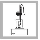
**20.** Stir the sample vigorously with the probe or use a stir stand and stir bar. When measuring deep bodies of water, create sufficient flow across the probe tip by pulling on the cable to move the probe up and down.
