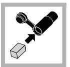
**5.** Prepare the calibration and storage chamber by holding it under water and squeezing it a couple of times to pull water into the lower chamber through the inlet.
