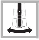
**19.** Agitate the probe in the sample to dislodge air bubbles from the sensing area of the probe tip.
