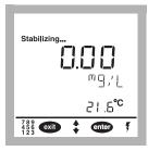
**3.** Zero the *sension*<sup>TM6</sup> Dissolved Oxygen meter prior to calibration when measuring dissolved oxygen levels less than 1 mg/L or 10% saturation.
