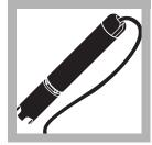
**16.** Add the weight assembly to the probe if required (3- or 15-m cable versions only).
