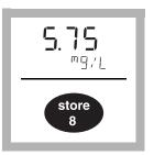
**21.** When the reading on the meter stabilizes, record or store the value in the meter memory.
