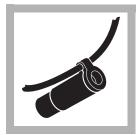
**4.** Secure the probe cable to the calibration and storage chamber by wrapping cable through the bottom of the chamber lid before filling with water.
