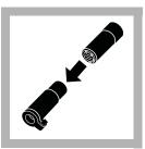
6. Insert the DO probe into the calibration and storage chamber. The probe tip must not be flooded with water or be holding a drop of water on the membrane.
