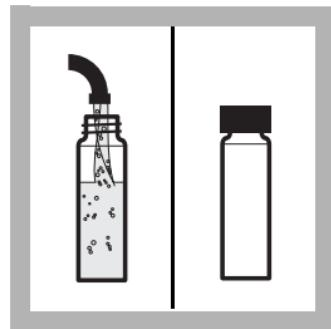
3. Rinse the bottle several times with sample water. The bottle is now ready for use in the test.
