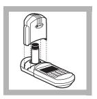
7. Wipe the outside of the sample cell with a towel. Place the blank into the cell holder. Tightly cover the sample cell with the instrument cap.
