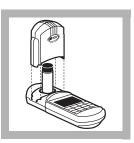
**7.** Place the blank into the cell holder. Tightly cover the sample cell with the instrument cap.
