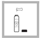
**4.** Add the contents of one NitriVer 3 Nitrite Reagent Powder Pillow to the sample cell. Cap the cell and shake to dissolve.
