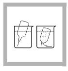
**3.** Collect at least 40 mL of sample in a 50-mL beaker. Fill a NitriVer 3 Nitrite AccuVac Ampul with the sample.
