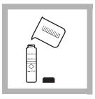
**6.** When the timer beeps, fill a sample cell with at least 10 mL of sample (the blank).
