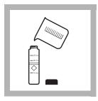
**6.** When the timer beeps, fill an empty sample cell with 10 mL of sample (the blank).
