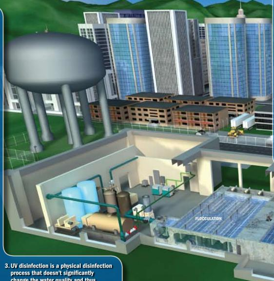
4. UV lamps are the most important components of UV disinfection equipment. Most lamps used in these systems are mercury vapor lamps, so operators should be trained in proper cleanup procedures in case a lamp breaks.
